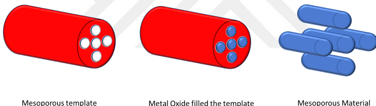
Figure 1.3.1 Three steps of hard templating method.
