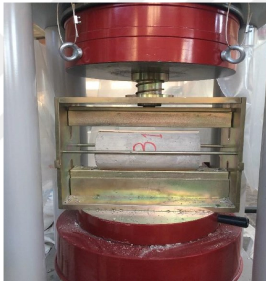
Figure 3.12 Brazilian indirect tensile test.
