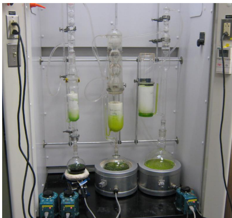
Figure 12. Soxhlet extraction model.
