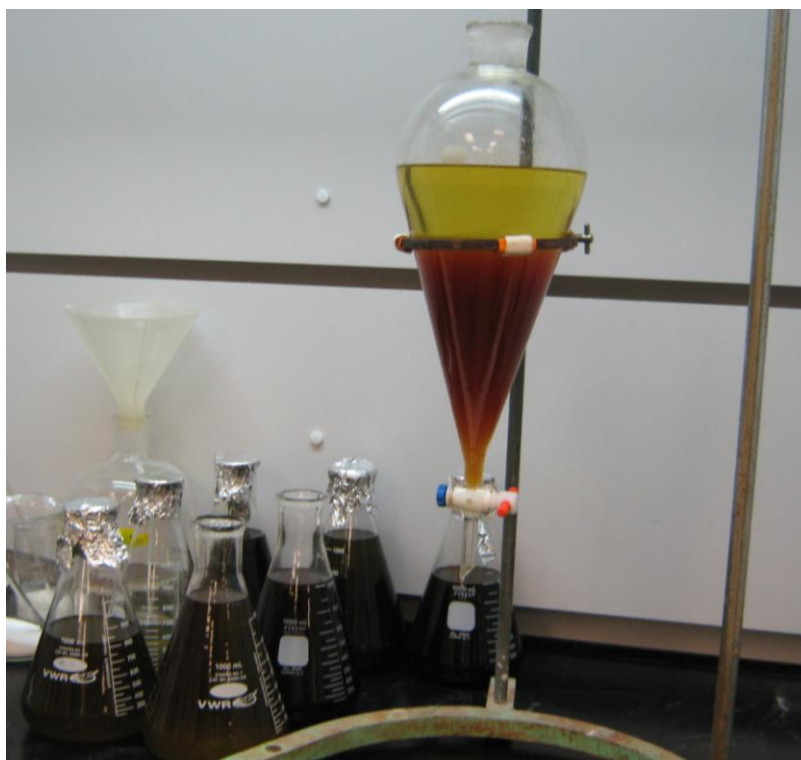
Figure 14. Liquid- liquid extraction model.
