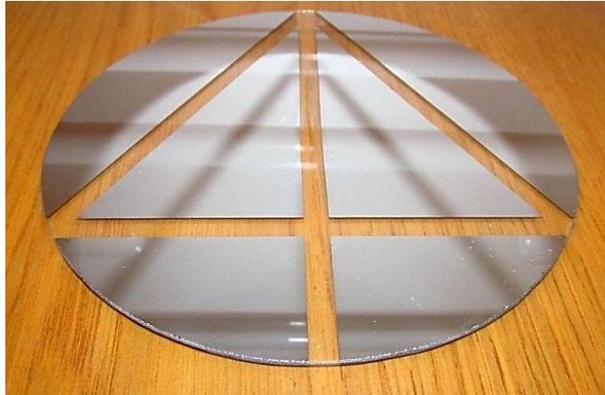
Figure 4.2. The view of plain glass substrate after removal of kapton tape.
