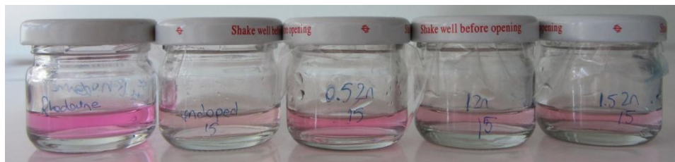
Figure 3.85. After 15 hours radiation (left to right: unradiated Rhodamine B, Rhodamine B belongs to undoped \text{TiO}_2 , 0.5 % Zn- \text{TiO}_2 , 1 % Zn- \text{TiO}_2 , 1.5 % Zn- \text{TiO}_2 )
