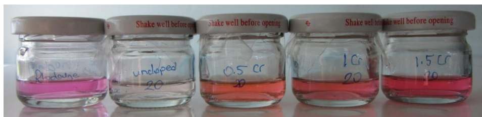
Figure 3.90. After 20 hours radiation (left to right: unradiated Rhodamine B, Rhodamine B belongs to undoped TiO 2 , 0.5 % Cr-TiO 2 , 1 % Cr-TiO 2 , 1.5 % Cr-TiO 2 )
