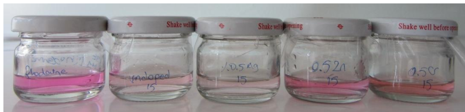
Figure 3.93. After 15 hours radiation (left to right: unradiated Rhodamine B, Rhodamine B belongs to undoped \text{TiO}_2 , 0.5 % Ag- \text{TiO}_2 , 0.5 % Zn- \text{TiO}_2 , 0.5 % Cr- \text{TiO}_2 )
