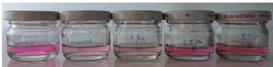
Figure 3.92. After 10 hours radiation (left to right: unradiated Rhodamine B, Rhodamine B belongs to undoped \text{TiO}_2 , 0.5 % Ag- \text{TiO}_2 , 0.5 % Zn- \text{TiO}_2 , 0.5 % Cr- \text{TiO}_2 )
