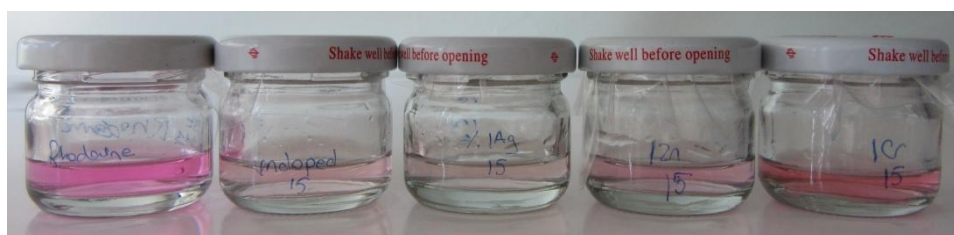
Figure 3.97. After 15 hours radiation (left to right: unradiated Rhodamine B, Rhodamine B belongs to undoped TiO 2 , 1 % Ag-TiO 2 , 1 % Zn-TiO 2 , 1 % Cr-TiO 2 )
