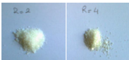
Figure 3.6. TiO 2 powders obtained by drying TiO 2 solutions (R=2, \frac{1}{2} propanol, R=4) at 50 °C
