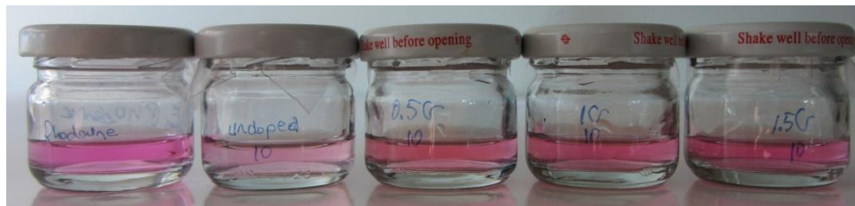
Figure 3.88. After 10 hours radiation (left to right: unradiated Rhodamine B, Rhodamine B belongs to undoped TiO 2 , 0.5 % Cr-TiO 2 , 1 % Cr-TiO 2 , 1.5 % Cr-TiO 2 )
