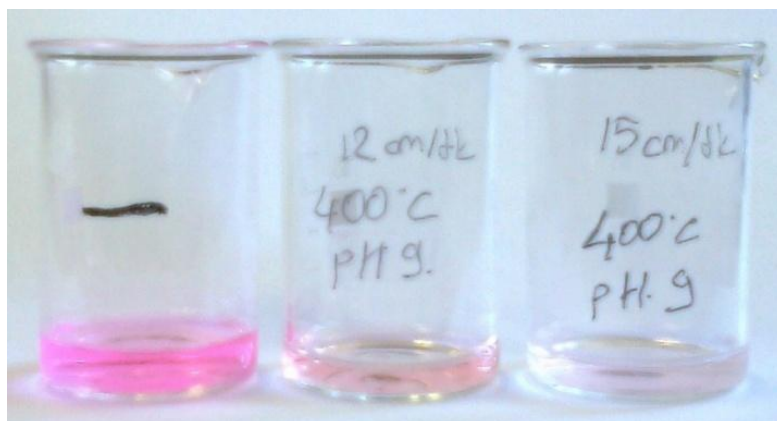
Figure 3.76. Rhodamine B solution after 15 hours radiation, sintering temperature=400 °C, pH of Rhodamine B solution=9. (left to right: unradiated Rhodamine B, Rhodamine B belongs to the SLS glass coated with a withdrawal speed of 12 cm/min, Rhodamine B belongs to the SLS glass coated with a withdrawal speed of 15 cm/min)
