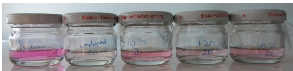
Figure 3.86. After 20 hours radiation (left to right: unradiated Rhodamine B, Rhodamine B belongs to undoped \text{TiO}_2 , 0.5 % Zn- \text{TiO}_2 , 1 % Zn- \text{TiO}_2 , 1.5 % Zn- \text{TiO}_2 )
