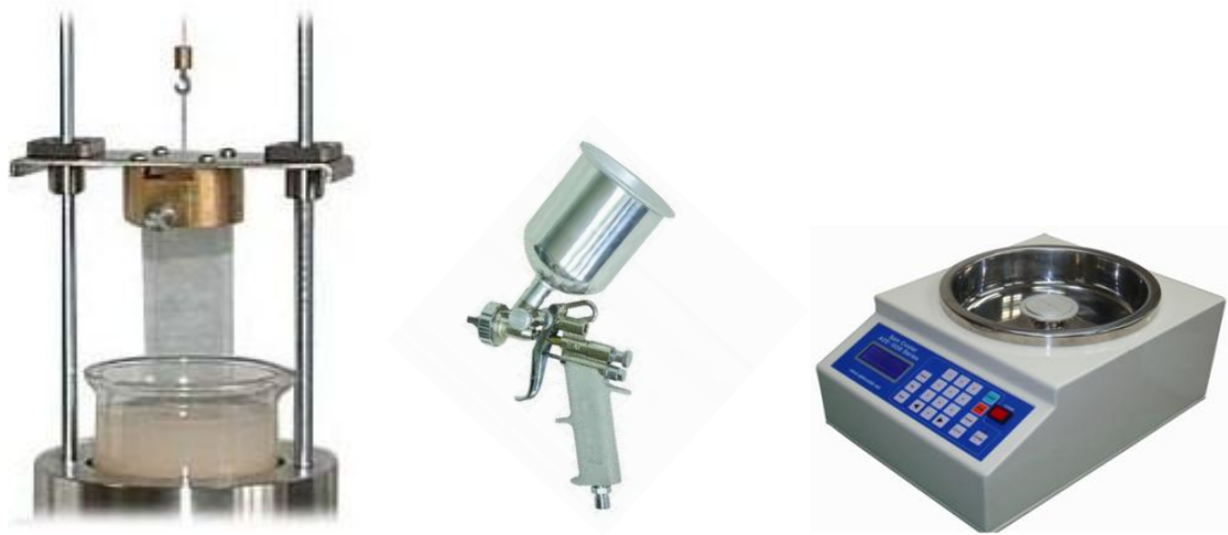
Figure 1.5. From left to right: Dip coater, Spray gun, spin coater
