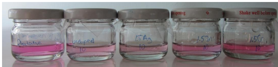
Figure 3.100. After 10 hours radiation (left to right: unradiated Rhodamine B, Rhodamine B belongs to undoped \text{TiO}_2 , 1.5 % Ag- \text{TiO}_2 , 1.5 % Zn- \text{TiO}_2 , 1.5 % Cr- \text{TiO}_2 )
