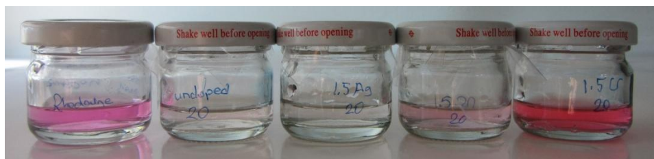
Figure 3.102. After 20 hours radiation (left to right: unradiated Rhodamine B, Rhodamine B belongs to undoped \text{TiO}_2 , 1.5 % Ag- \text{TiO}_2 , 1.5 % Zn- \text{TiO}_2 , 1.5 % Cr- \text{TiO}_2 )
