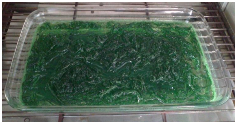
Figure 3.20. Gel of 1 % Cr doped \text{TiO}_2 obtained in oven at 33 °C
