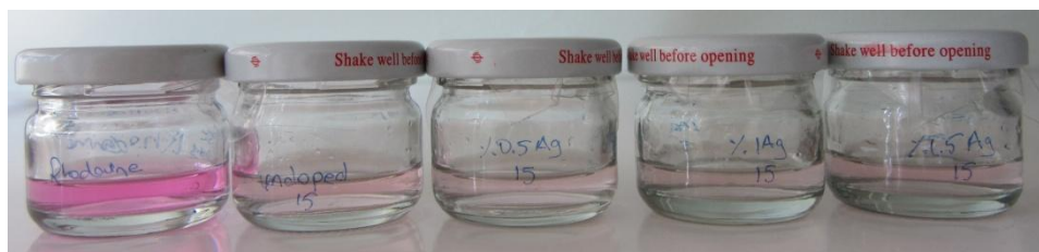
Figure 3.81. After 15 hours radiation (left to right: unradiated Rhodamine B, Rhodamine B belongs to undoped \text{TiO}_2 , 0.5 % Ag- \text{TiO}_2 , 1 % Ag- \text{TiO}_2 , 1.5 % Ag- \text{TiO}_2 )
