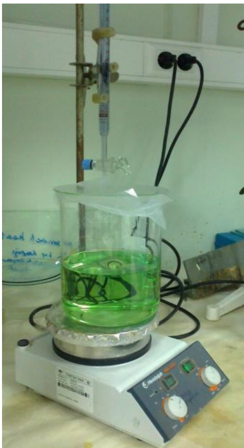
Figure 3.19. Preparation of 1 % Cr doped TiO 2 solution
