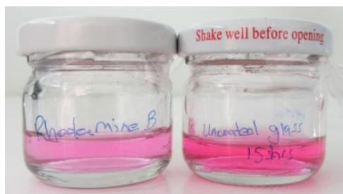
Figure 3.77. Unradiated Rhodamine B and Rhodamine B in which uncoated SLS glass is radiated for 15 hours.
