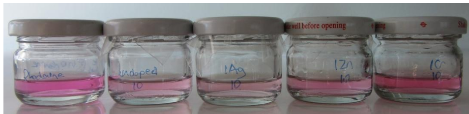
Figure 3.96. After 10 hours radiation (left to right: unradiated Rhodamine B, Rhodamine B belongs to undoped TiO 2 , 1 % Ag-TiO 2 , 1 % Zn-TiO 2 , 1 % Cr-TiO 2 )
