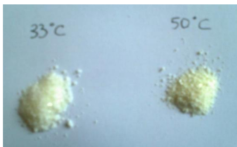
Figure 3.2. \text{TiO}_2 powders obtained by drying \text{TiO}_2 solutions (R=2) at 33 °C and 50 °C
