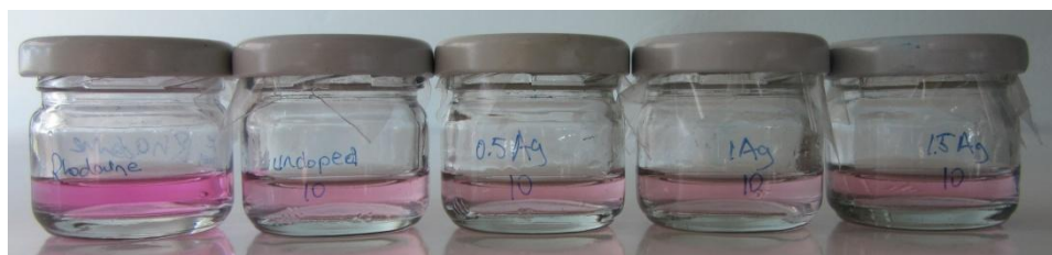
Figure 3.80. After 10 hours radiation (left to right: unradiated Rhodamine B, Rhodamine B belongs to undoped \text{TiO}_2 , 0.5 % Ag- \text{TiO}_2 , 1 % Ag- \text{TiO}_2 , 1.5 % Ag- \text{TiO}_2 )
