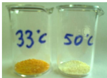
Figure 3.3. TiO 2 powders after moisture removal at 100 °C
