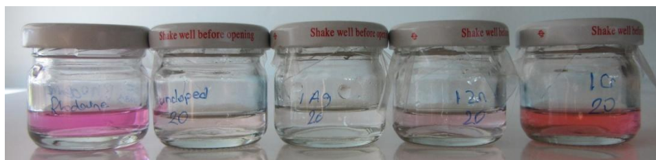
Figure 3.98. After 20 hours radiation (left to right: unradiated Rhodamine B, Rhodamine B belongs to undoped TiO 2 , 1 % Ag-TiO 2 , 1 % Zn-TiO 2 , 1 % Cr-TiO 2 )
