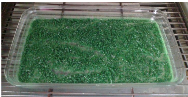
Figure 3.21. Powder of 1 % Cr doped \text{TiO}_2 obtained in oven at 33 °C
