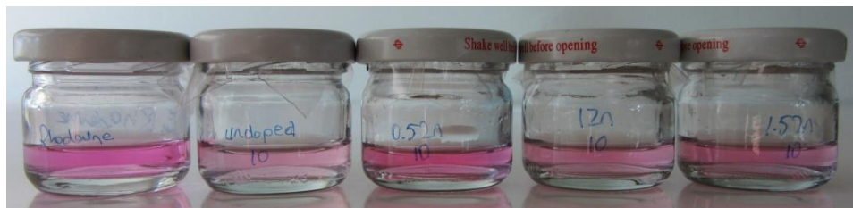
Figure 3.84. After 10 hours radiation (left to right: unradiated Rhodamine B, Rhodamine B belongs to undoped \text{TiO}_2 , 0.5 % Zn- \text{TiO}_2 , 1 % Zn- \text{TiO}_2 , 1.5 % Zn- \text{TiO}_2 )
