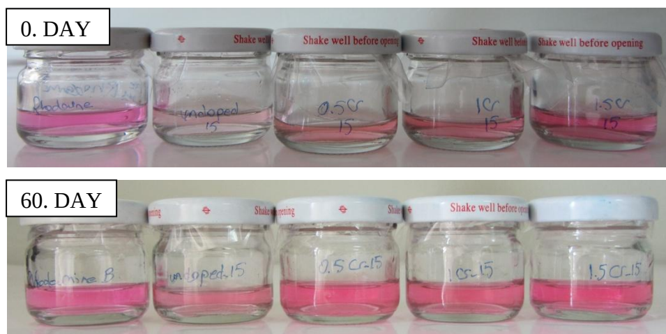
Figure 3.134. Comparison of photocatalytic activity of SLS glasses coated with Cr-TiO 2 at the 0 th and the 60 th day of preparation (left to right: unirradiated Rhodamine B, Rhodamine B belongs to undoped TiO 2 , 0.5 % Cr-TiO 2 , 1 % Cr-TiO 2 , 1.5 % Cr-TiO 2 )
