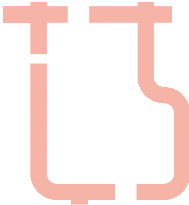
Figure 4.7: Momentum layout view of transmission lines connected to the gates and drains of the two transistors.
