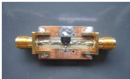
Figure 4.1: Fixture for testing the transistors before mounting on the main board.
