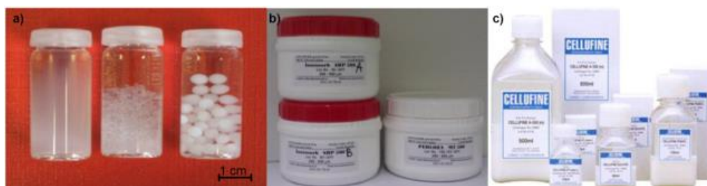
Figure 1.5. Different sizes of cellulose microspheres (a) and commercial cellulose microspheres (b, c). 18
