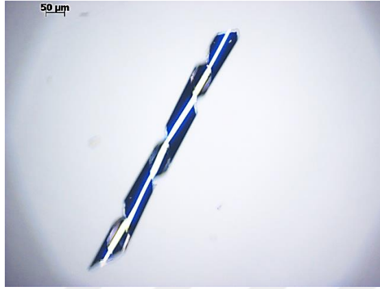
Fig. 3.14. The new swimmer with 150 nm sandwich nickel
