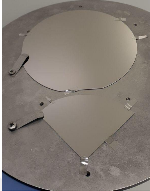
Fig. 2.8. Nickel thin film deposited by E-beam PVD on LF Silicon nitride
