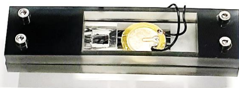
Fig. 2.27. The glass-PDMS-transducer setup
