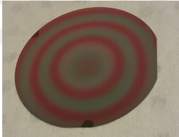
Fig. 2.13. Wafer coated with 1.4 \mu\text{m} PR
