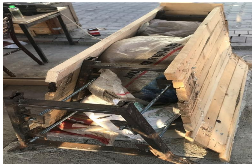
Figure 3.6. Arrangement of sandbags of hybrid barrier.
