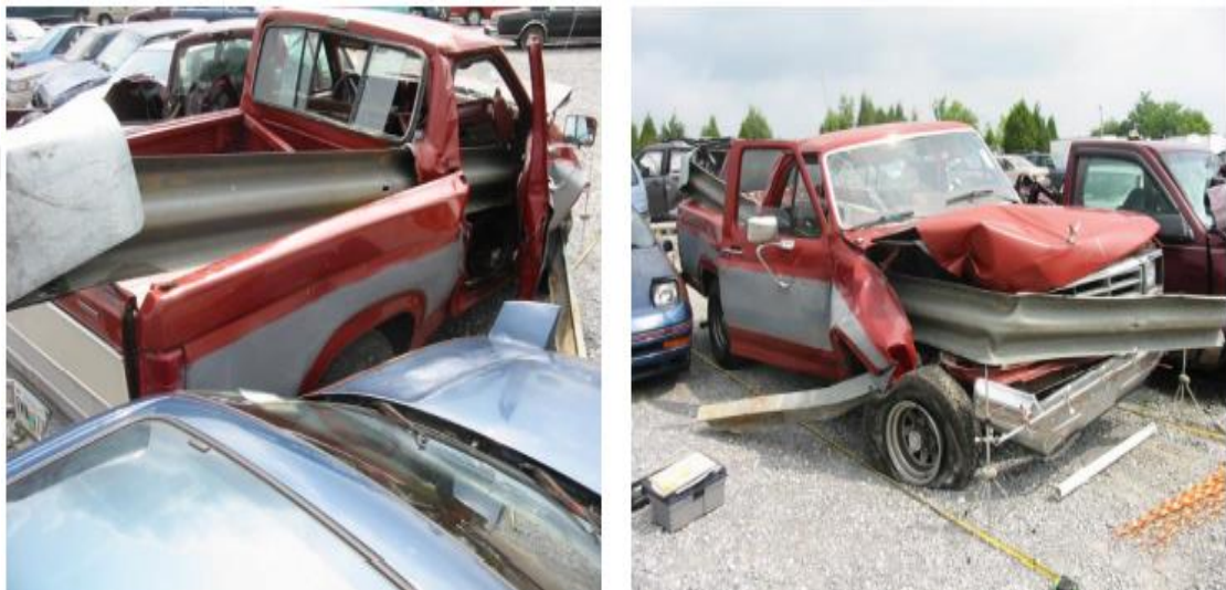
Figure 2.5. Guardrail penetrated the vehicle [59].
