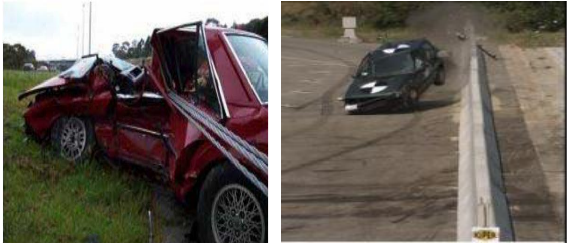
Figure 1.2. Accident crash of cable, guardrail and concrete barrier [8,12,14].
