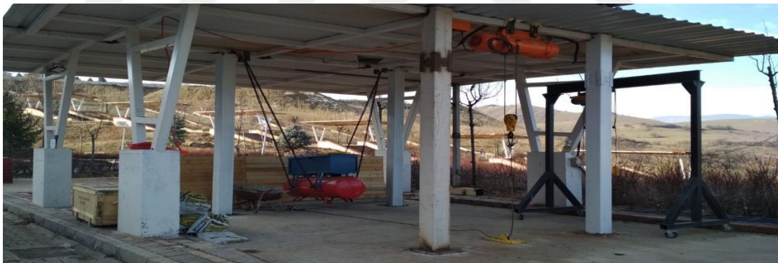
Figure 4.4. (a) Pendulum rammer and (b) Electric chain pulley
