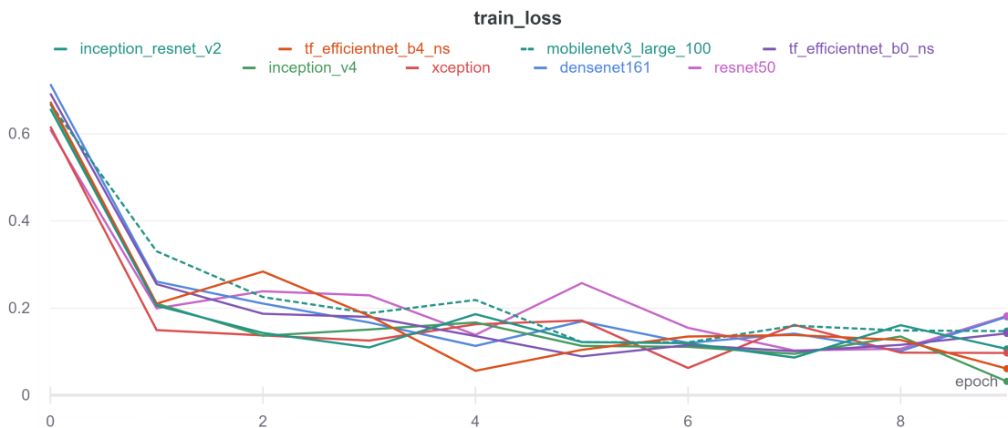
Figure 2.13 Train loss over epochs of the models trained with fixed Learning rate and default augmentation setup.
