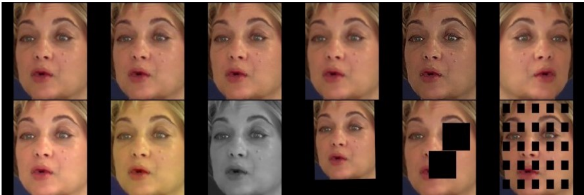
Figure 2.12 Augmentations: From top left: Source image, compression, Gauss noise, blur, sharpening, horizontal flip, brightness, hue and saturation value adjustment, gray, shift+scale+rotate, Coarse dropout (size=64 pixels), Grid dropout. All images resized to 224 by preserving aspect ratio and padded with 0 value before an augmentation was applied.
