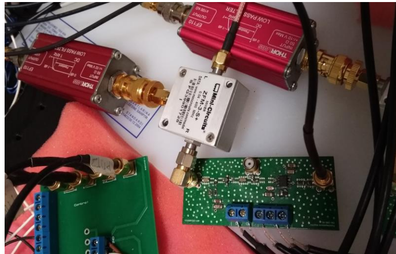
Figure 2.50. The implementation of four-layer multi-stage TIA
