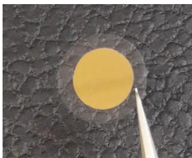
Figure 3.1: Au coated SPR chip. The diameter of Au coated area is 10 mm.
