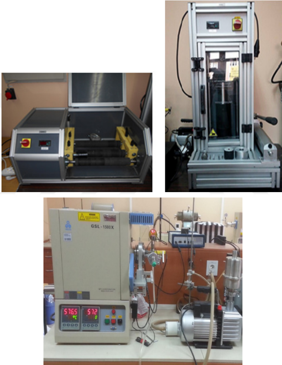
Figure 2.7: a) Ball mill and hydraulic press, b) sintering furnace
