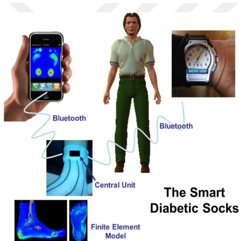
Figure 1.2 : Working mechanism of the design [4].
