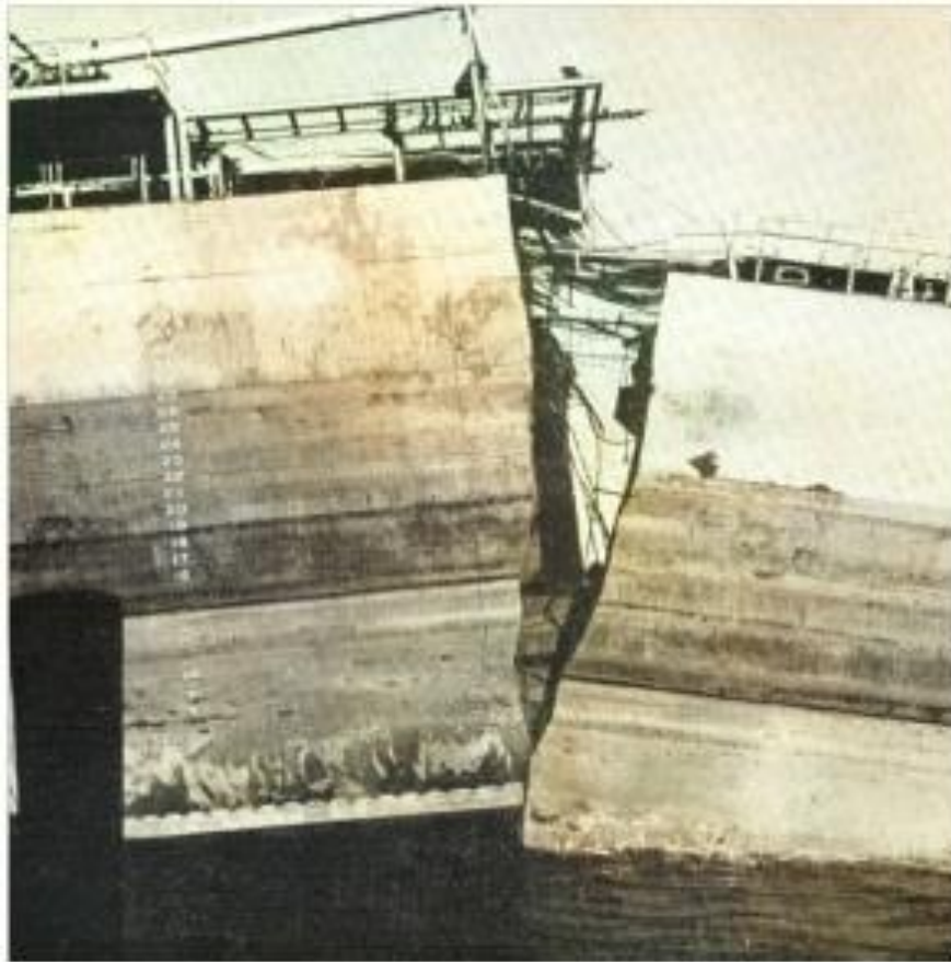
Figure 2.32. Fracture failure of Liberty ship [101]
