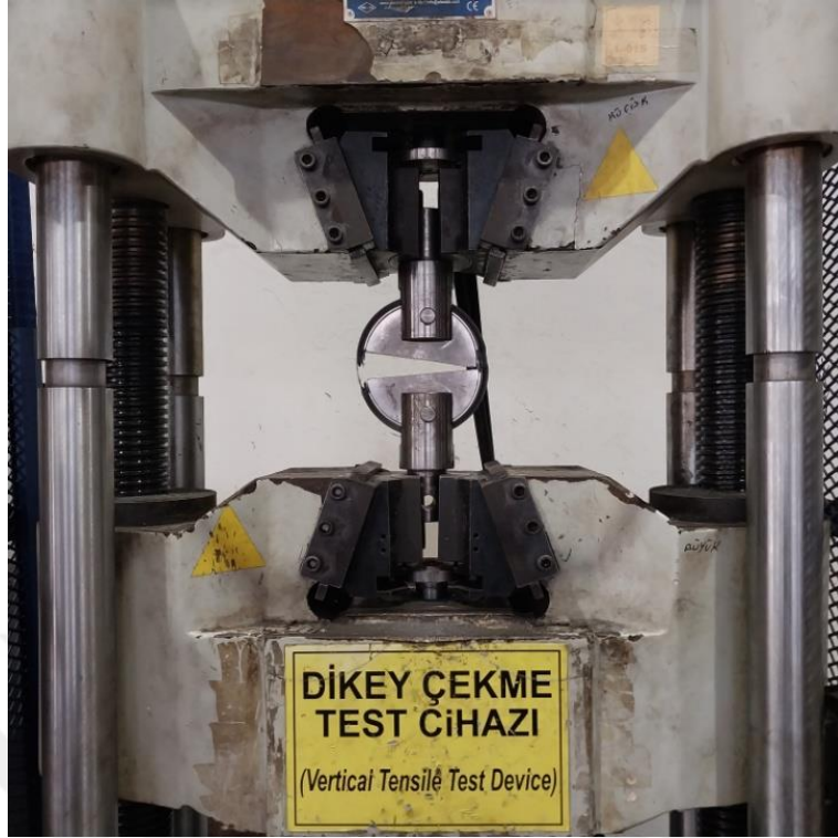
Figure 4.2. Failure of SDT specimen after tensile test
