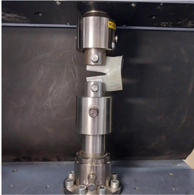
Figure 4.22. CCT specimen under load application
