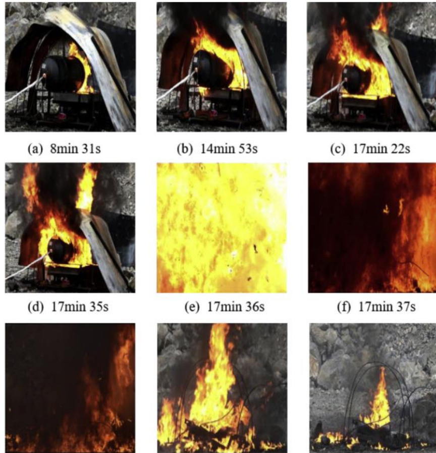
Figure 2.30. Fire explosion test of a type III tank [46]
