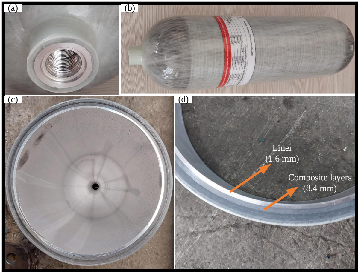
Figure 3.2. The type III composite tank: (a) the inlet port, (b) overview of the tank, (c) the inner of the tank, (d) the magnified view of the liner and composite layers
