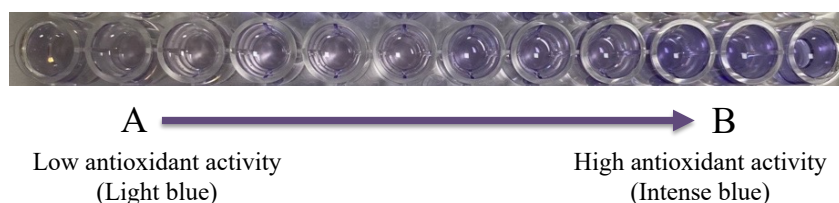
Figure 16. The color change occurred as a result of FRAP assay. A → B: Antioxidant activity from lowest to highest.
