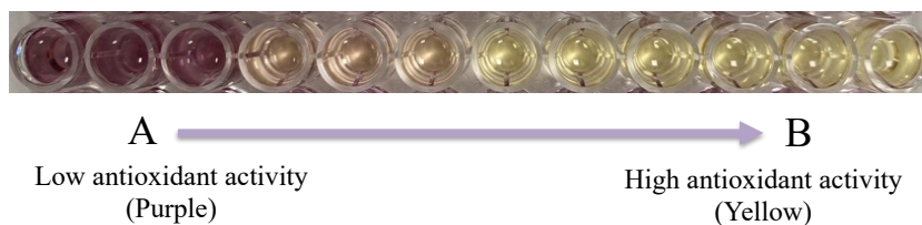
Figure 14. Discoloration of the DPPH reagent. A → B: Antioxidant activity from lowest to highest.
