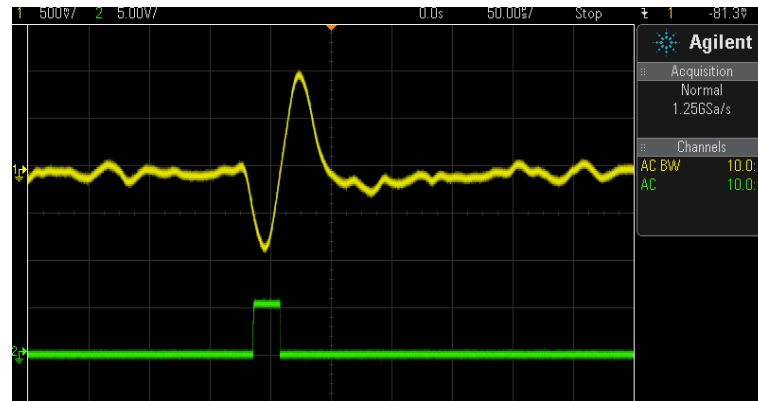
Figure 3.5 : An Analog and the Digital Signals from ^{137}\text{Cs} 662 keV gamma
