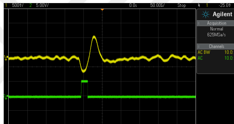
Figure 3.6 : An Analog and the Digital Signals from ^{241}\text{Am} 59 keV gamma
