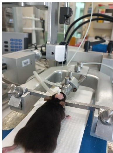
Figure 20. Placement of an optic ferule on the head of mice for Optogenetic stimulation.
