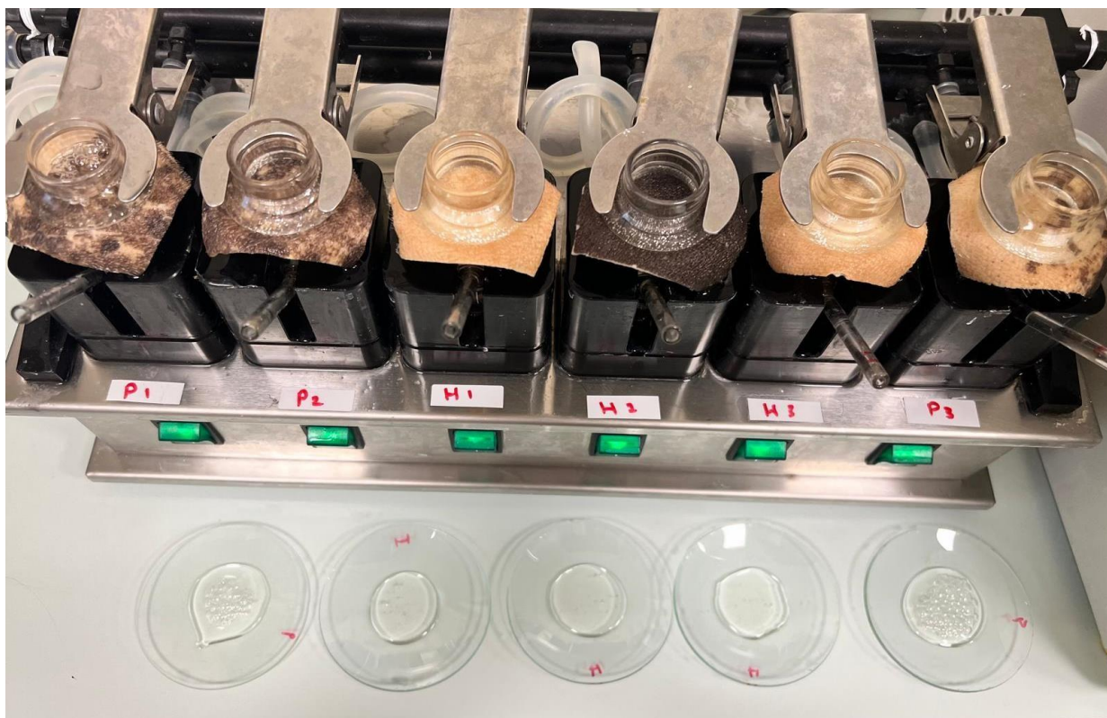
Figure 2.2.5. Franz diffusion cells set up Naproxen sodium gel formulations.
