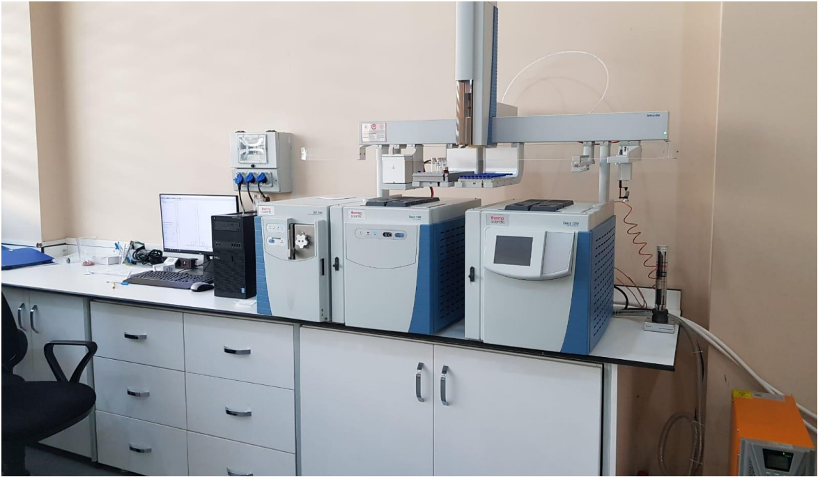
Şekil 3.7. Analizlerde kullanılan head space GC-MS cihazı [Triplus HS Autosampler, Thermo Scientific Trace 1300 GC, Thermo Scientific- ISQ7000 single Quadrupole Mass Spectrometer (Thermo Fisher Scientific Inc. Waltham, Massachusetts, ABD)]
