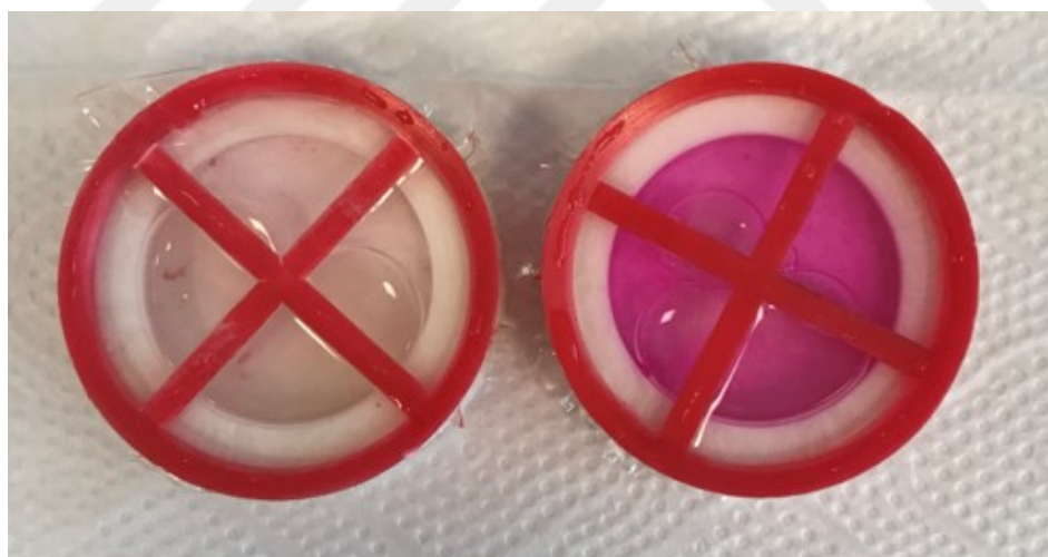
Figure 3-11 : The photograph of drug release capsules at pH=7.4(left) and pH=5.0 (right) after 72h at 40°C
