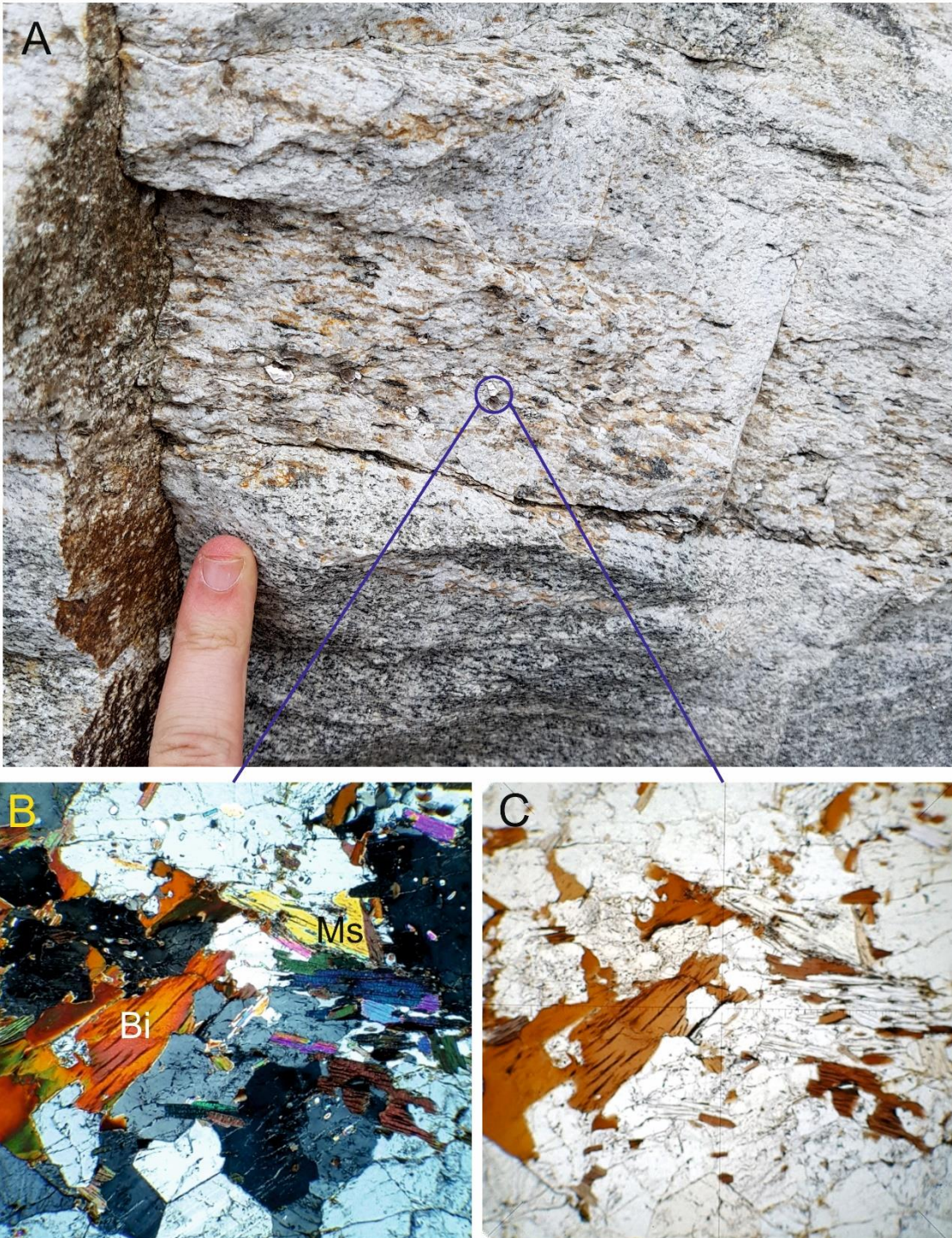
Figure 4.5 : Two-mica granite in field and microphotographs under cross-polarized light (b) and plane-polarized light (c). Magnification of thin section photographs: 4X.
