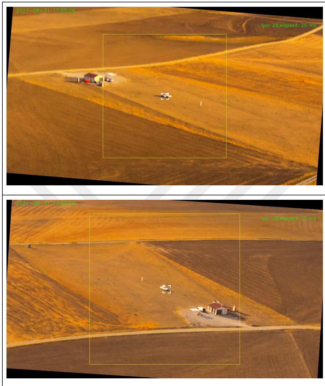
Figure 5-9: Successive target tracking and image-based loitering.
