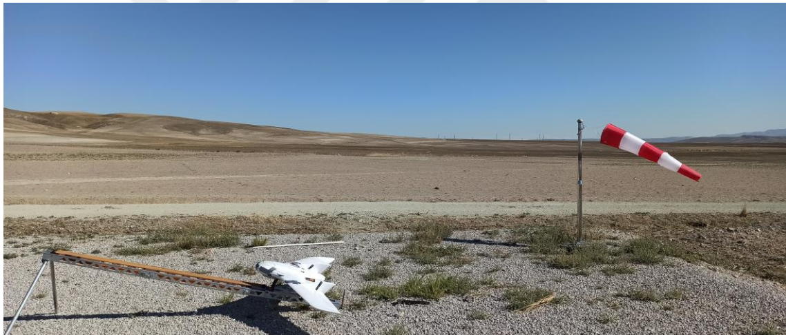
Figure 3-1: Flight test setup, UAV and the launcher
