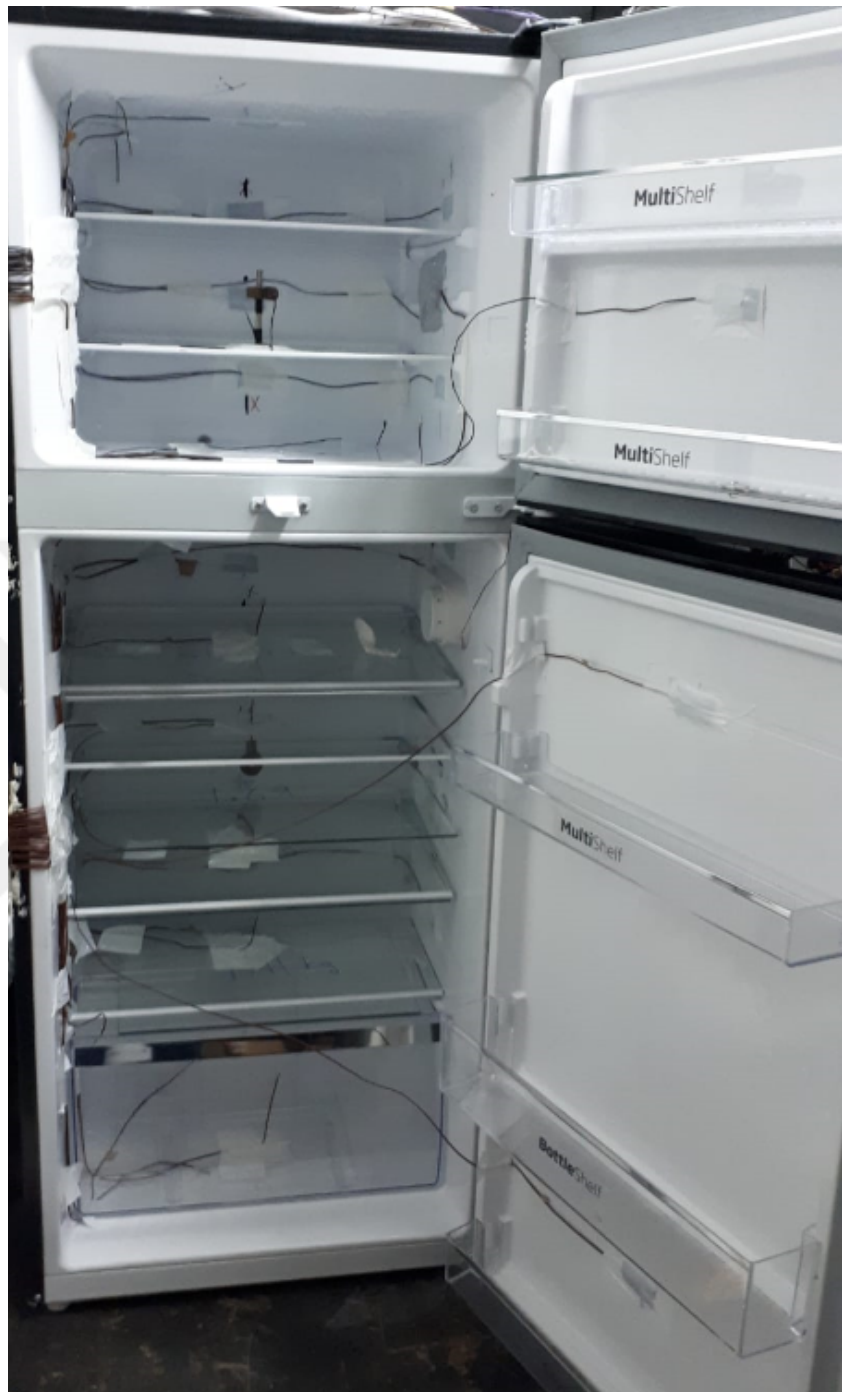
Figure 6.8. Thermocouples placed inside both compartments.
