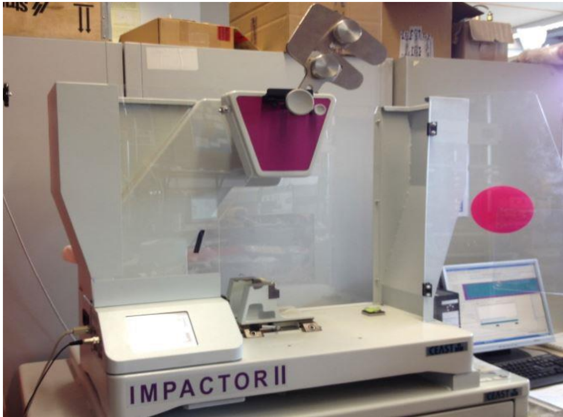
Figure 4. 2 The test machine utilized in NbZr impact deformation.
