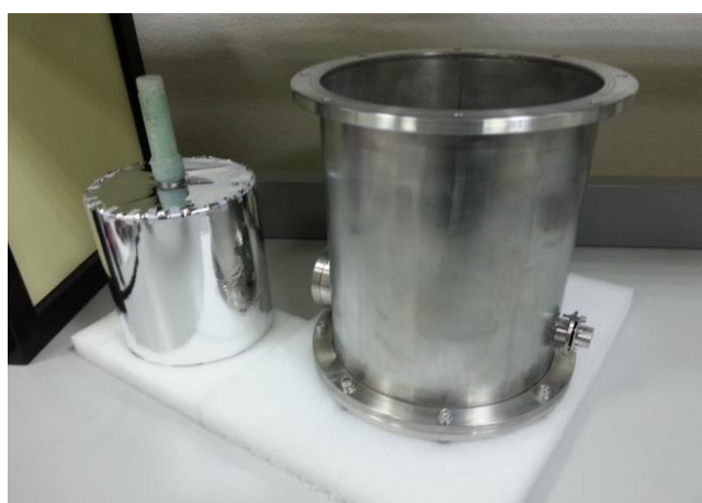
Figure 3.22. Liquid nitrogen reservoir coated with metallized film
