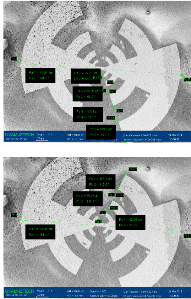
Figure 4.5. SEM images of antenna with dimensions on Bi2212 thin film
