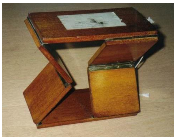
Figure 5.7. 6R Sarrus Mechanism (Source: Chen, 2003)
