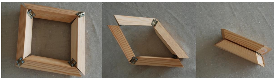
Figure 5.13. Bennett linkage with skew square cross-section bars
