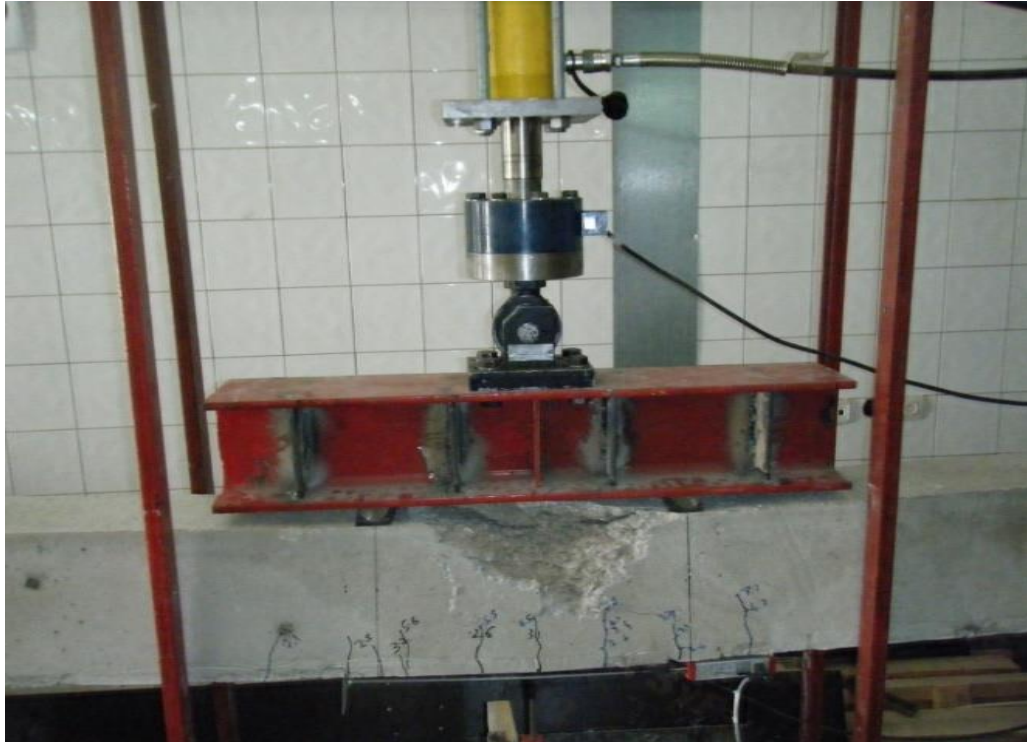
Figure 4-9 – Failure and crack pattern in a PC Beam 3φ18 ( \rho = 2.02\% )
