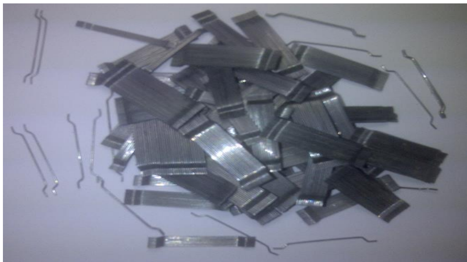
Figure 3-3 – Dramix ZP 305 steel fiber used in the research
