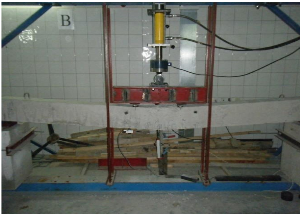
Figure 4-3 – Failure and crack pattern in SFRC Beam 3φ20 ( \rho = 2.50\% )
