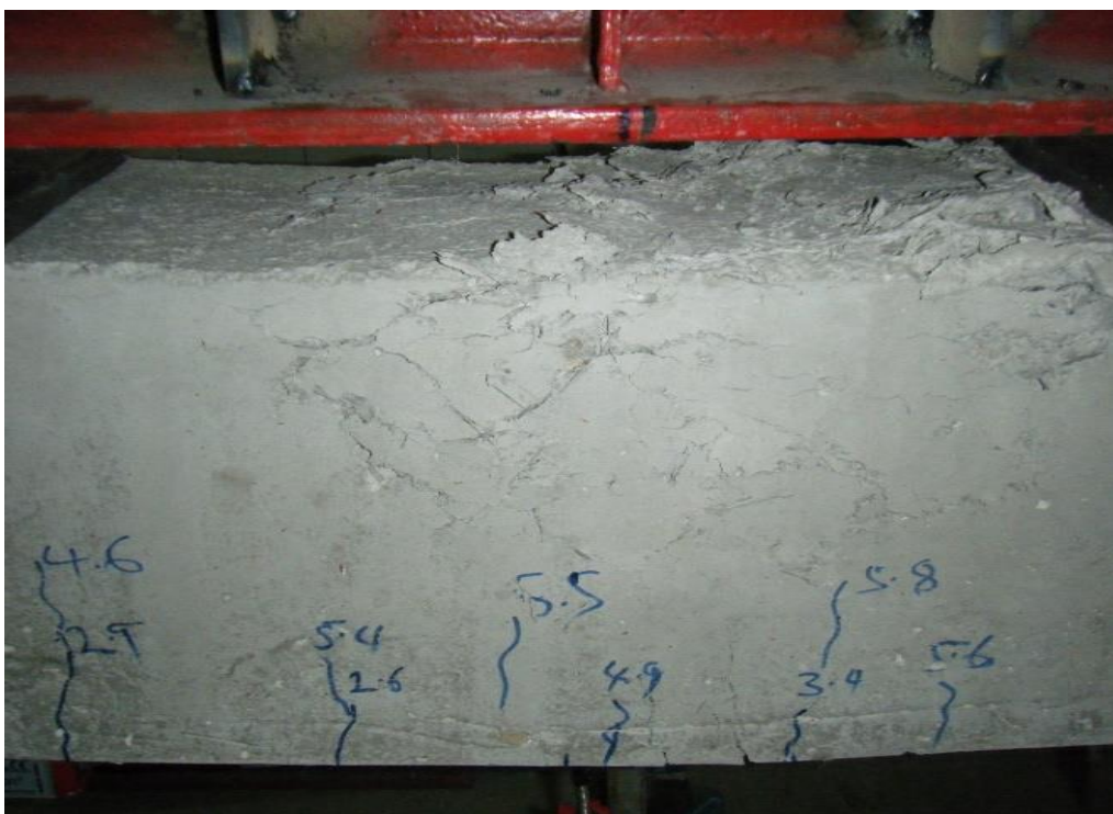
Figure 4-4 – Failure and crack pattern in SFRC Beam 3φ20 ( \rho = 2.50\% )
