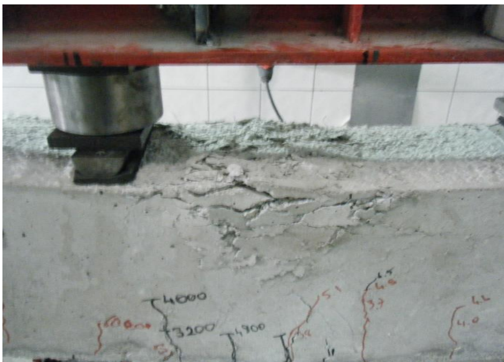
Figure 4-8 – Failure and crack pattern in SFRC Beam 4 \phi 16 ( \rho = 2.13\% )
