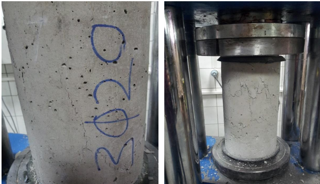
Figure 4-1 – Failure mode of concrete cylinders for SFRC Beam 3 \phi 20
