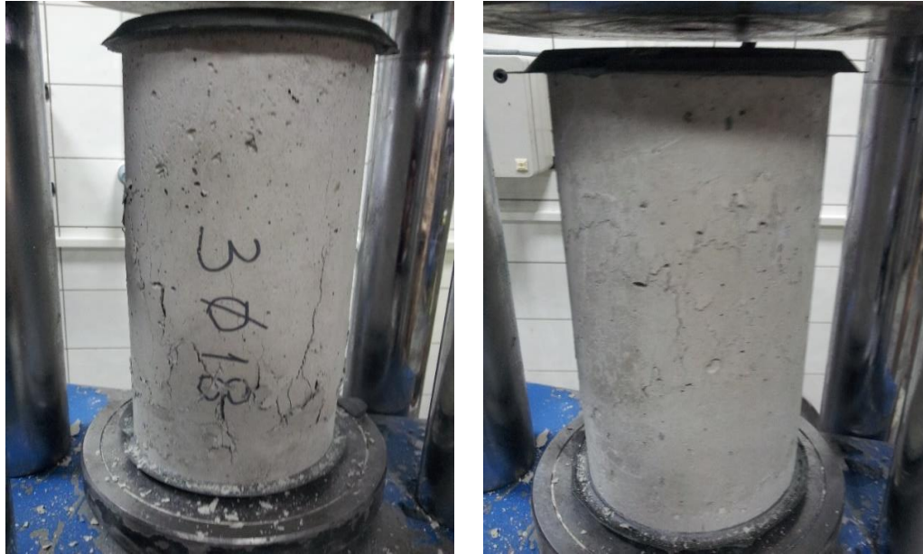
Figure 4-2 – Failure mode of concrete cylinders for SFRC Beam 3φ18
