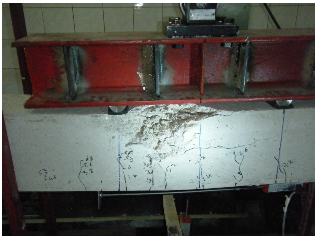
Figure 4-10 – Failure and crack pattern in a PC Beam 4φ16 ( \rho = 2.13\% )
