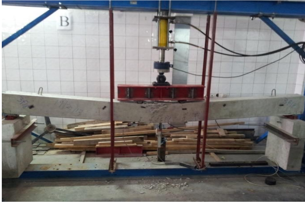
Figure 4-5 – Failure and crack pattern in SFRC Beam 3φ18 ( \rho = 2.02\% )
