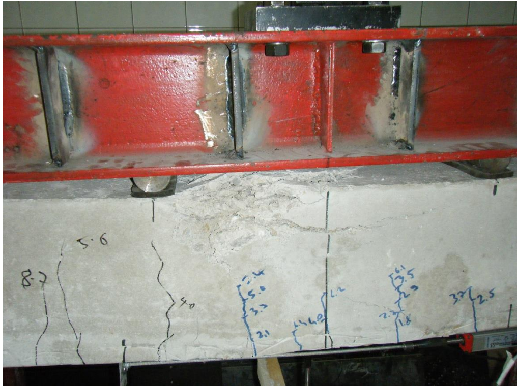
Figure 4-11 – Failure and crack pattern in a PC Beam 3 \phi 20 ( \rho = 2.50\% )
