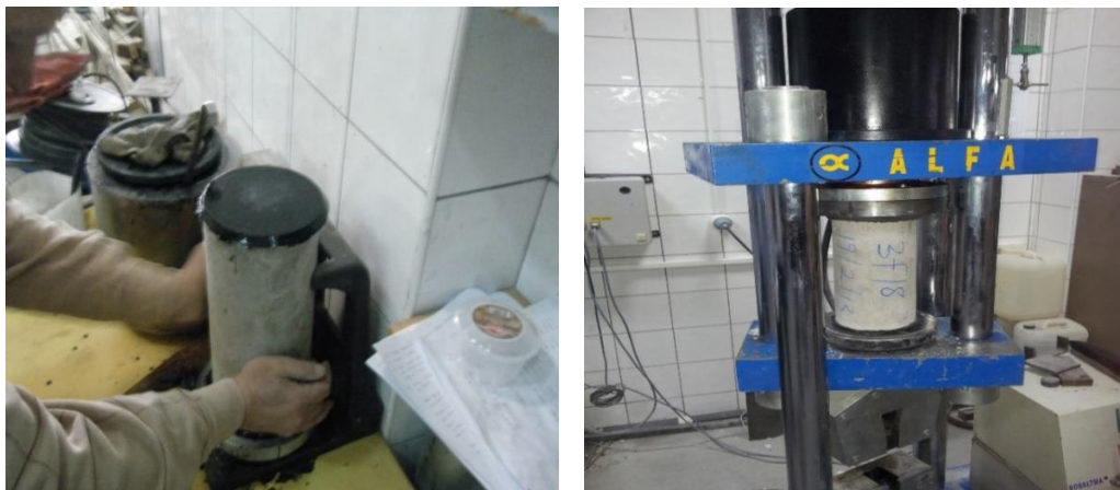
Figure 3-9 – Capping and testing of cylinder samples
