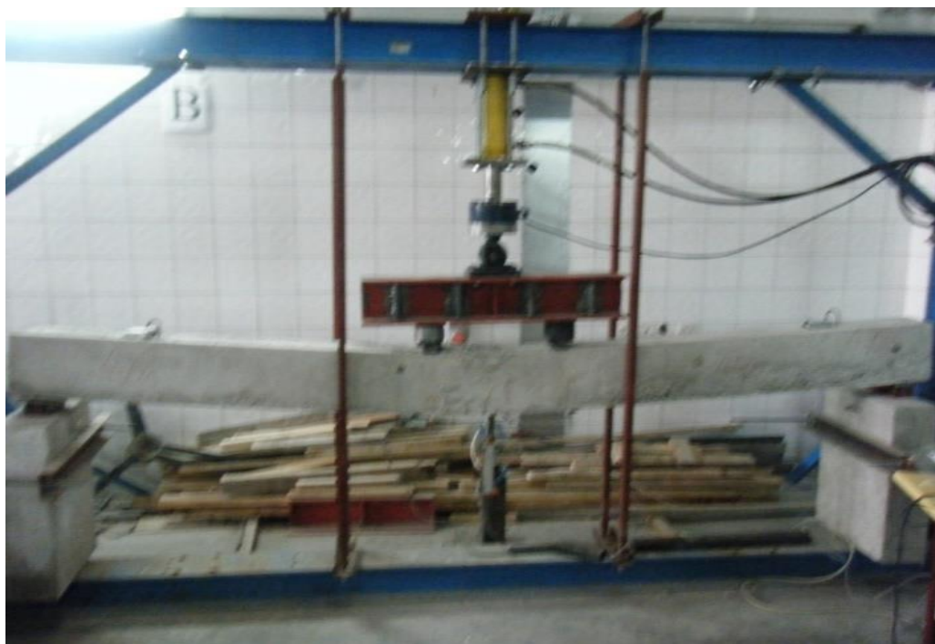
Figure 4-7 – Failure and crack pattern in SFRC Beam 4 \phi 16 ( \rho = 2.13\% )
