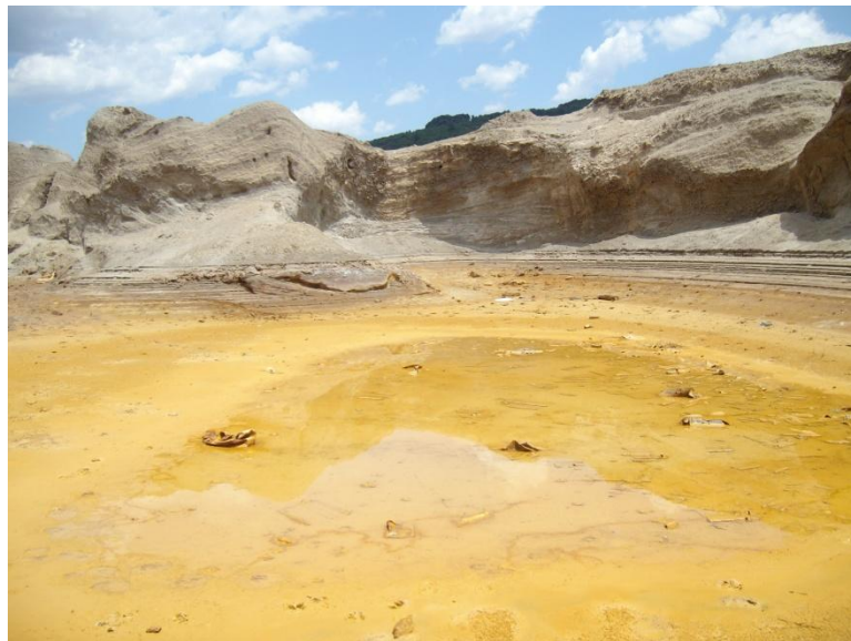
Figure 1.6: Acid mine water in the Balya Pb-Zn tailing area
