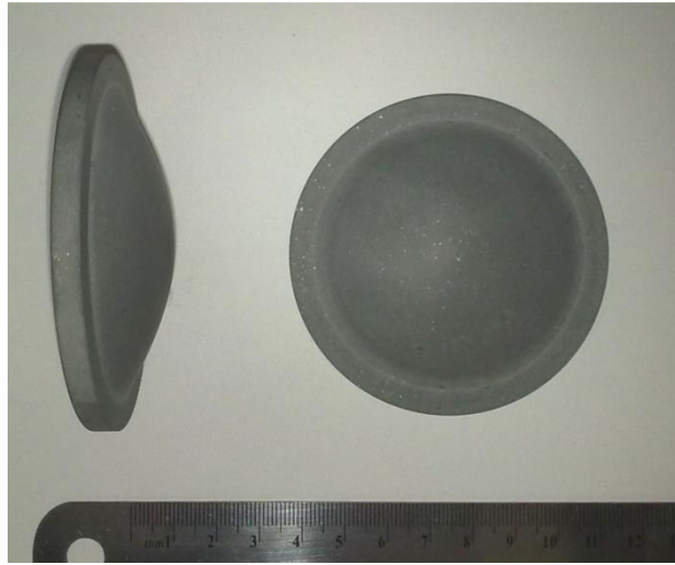
Figure 3.9 Polymeric lenses used in free-space measurement system.
