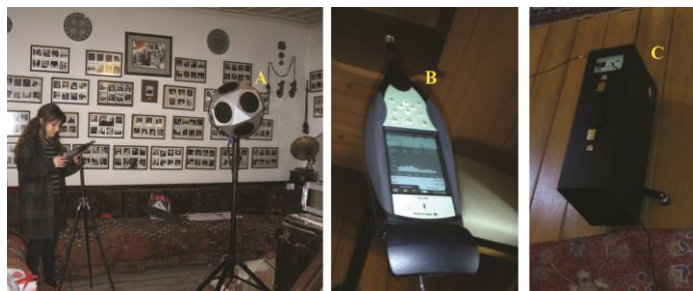
Figure 3.27 Instruments of in-situ acoustical measurements. A: omnidirectional sound source; B: sound level meter; C: tapping machine.
