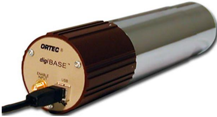
Figure 3.3 Ortec digiBASE and 3''x3'' NaI(Tl) detector [24]
