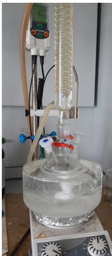
Figure 3.3: Experimental set-up of emulsion polymerization
