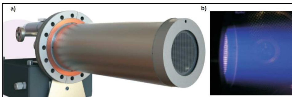
Figure 3.3 a) RF Ion Source and b) Argon Plasma [63,64].
