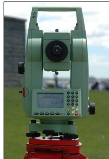
Fig.2.5. A reflectorless Total Station, LEICA TCR702, DSOL, June 2006.
