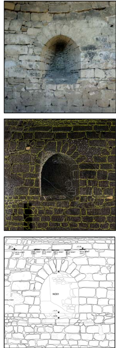
Fig. 5. 6. From the scan data to the CAD drawings, the Seddülbahir Project.
