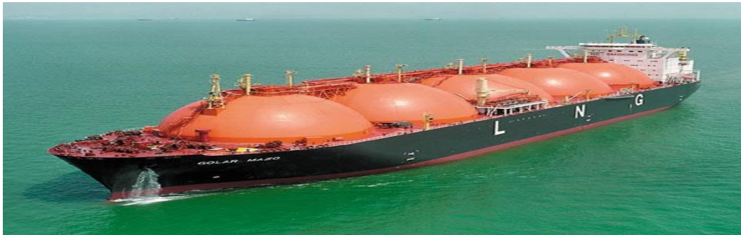
Figure 2.3: LNG ship with spherical Moss-Rosenberg tanks. Source: Url-14 .
