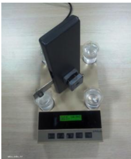
Figure 3.6. The image of SILAR setup used in the experiments.
