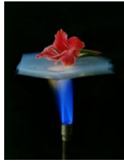
Figure 2.6. Superinsulating property of silica aerogel [15]
