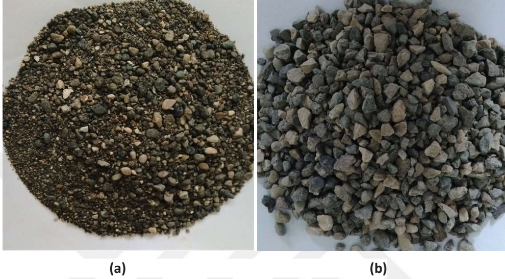
Şekil 2. (a) 0-4 mm agregaya, (b) 4-8 mm agregaya
