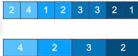
Figure 3.6. An exemplary maximum pooling operation with kernel size=2 and stride=2
