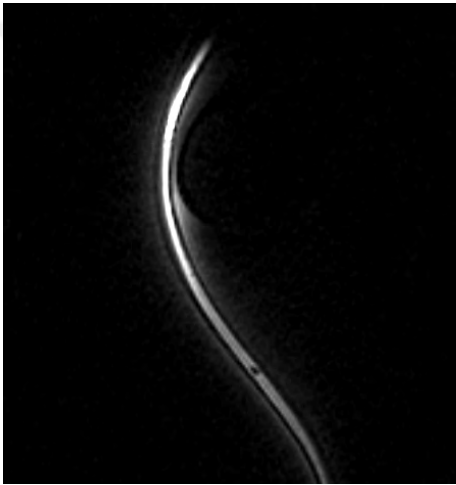
Figure 1.1: Projection image of a loopless catheter antenna placed in water. Imaging parameters are SPGR, 32 cm FOV, TR/TE = 5.2/1.5, 256x256 data acquisition matrix, 1 degree FA, 0 dB TG, no slice selection. Temporal resolution 1.3 s (5.2 ms x 256)
