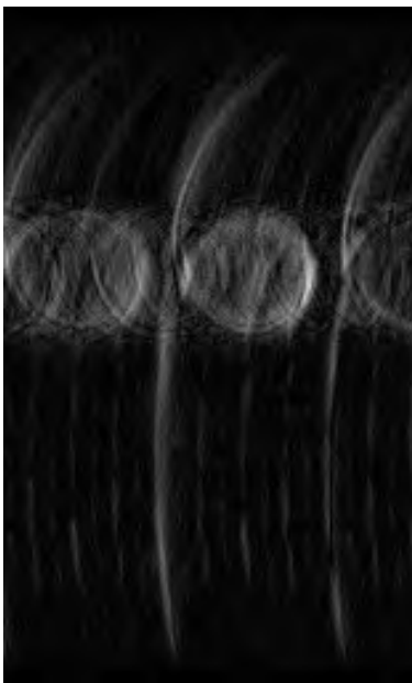
Figure 6.1: Full FOV image of a looped catheter. (Imaging parameters: FGRE, 256 \times 256 data matrix, 4^\circ FA, 0dB TG, 62.5kHz BW, TR/TE: 5.1/1.6msec, no slice selection)
