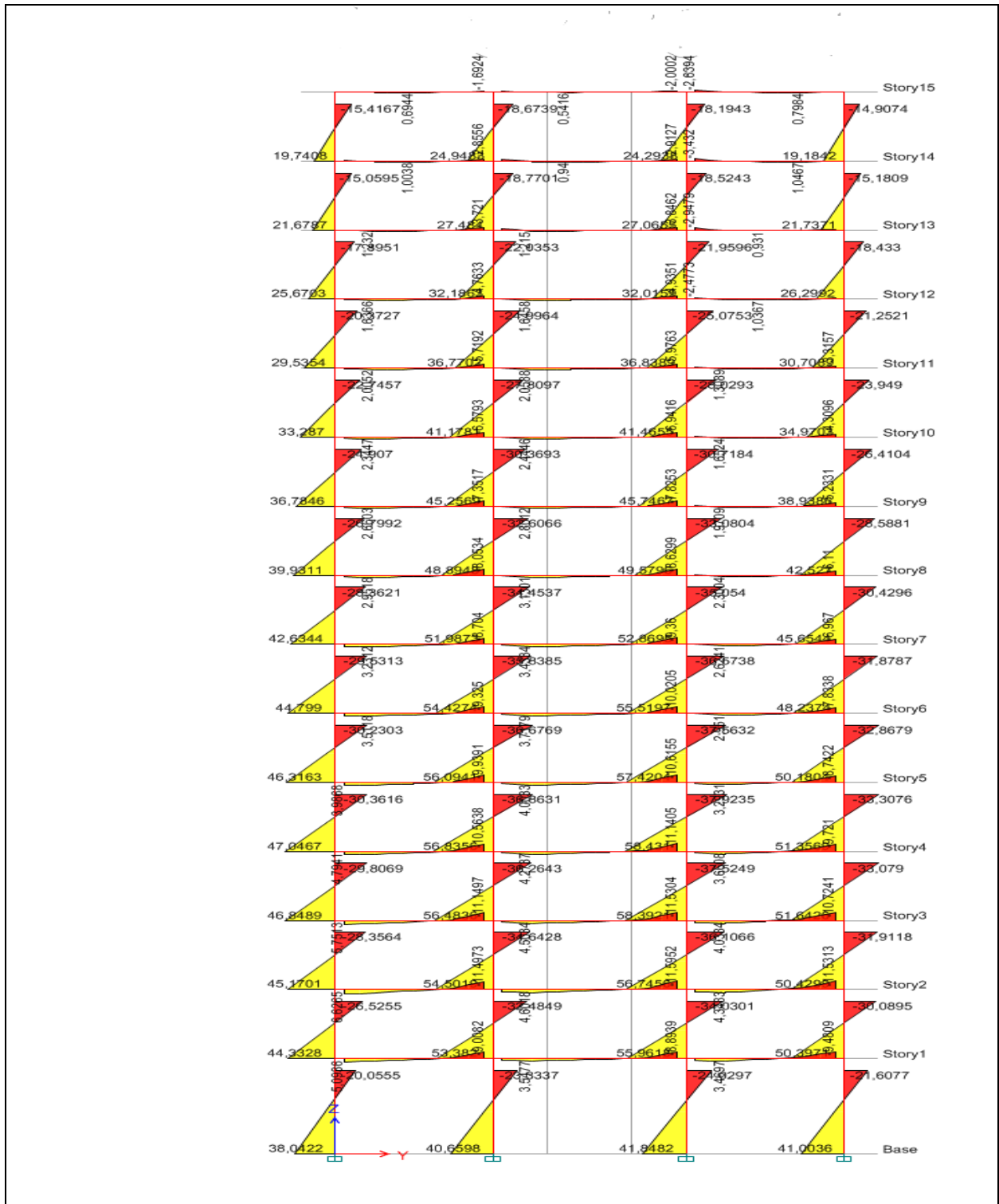
Figure 3.25: Bending Moment Diagram of Frame
