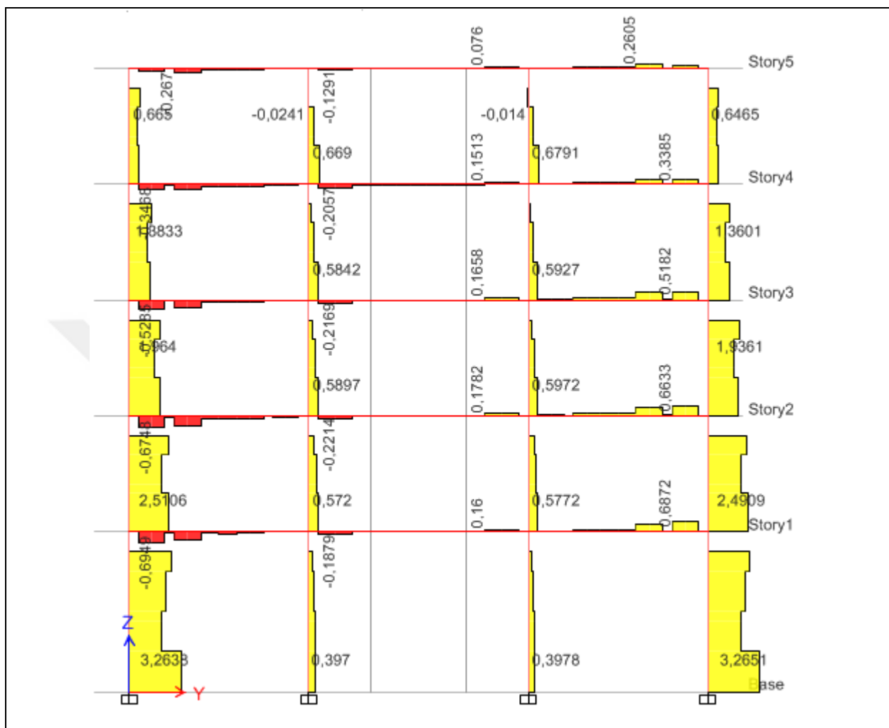
Figure 3.7: Shear Force Diagram of Frame
