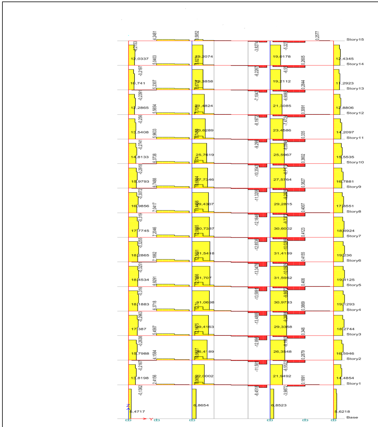
Figure 3.40: Shear Force Diagram of Frame
