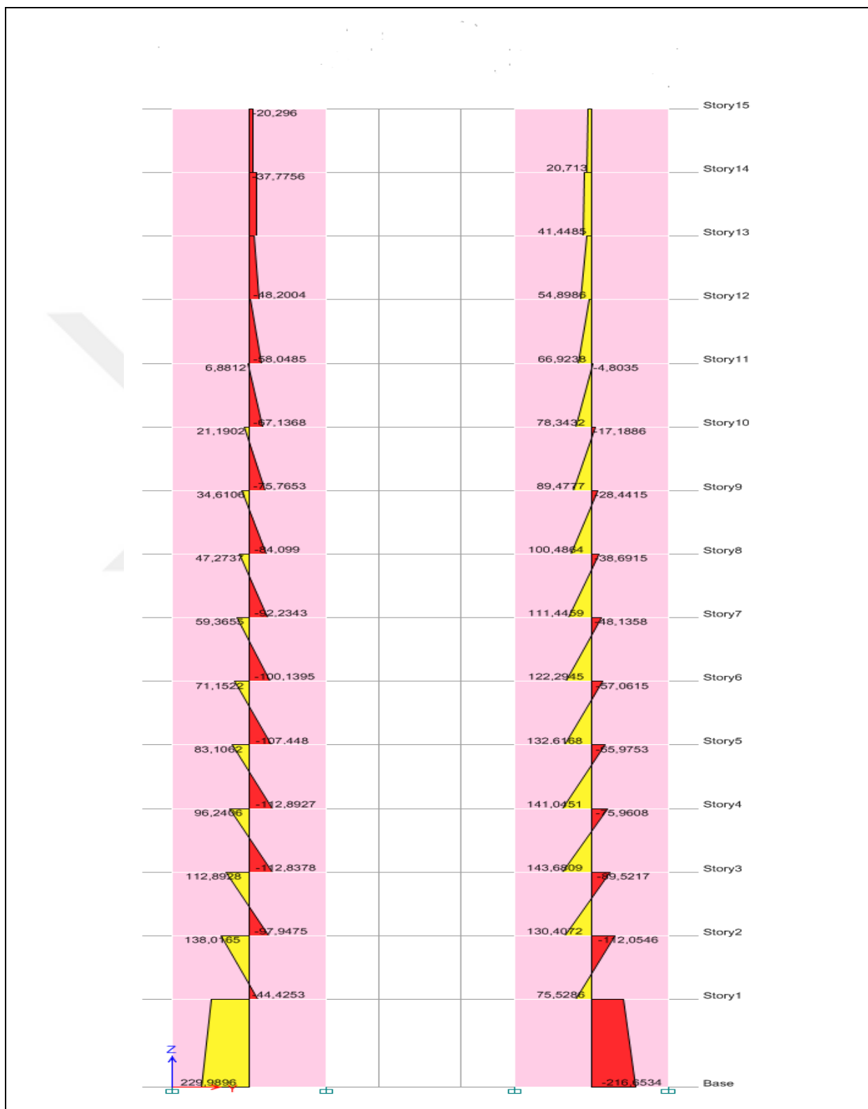
Figure 3.29: Bending Moment of Shear Wall
