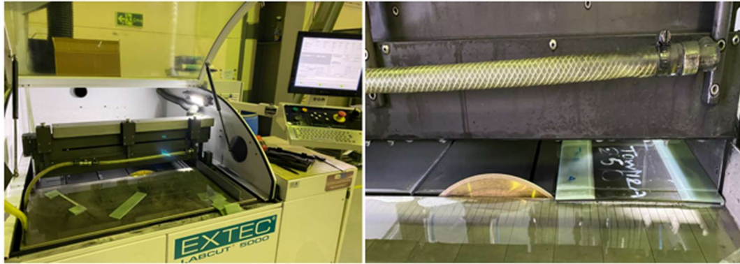
Figure 2.4 Machining of coupon specimens from the composite flat plates by using a precise wet machining system.
