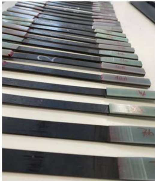
Figure 2.6 Schematic and images of the unidirectional tensile test specimen after tabbing.
