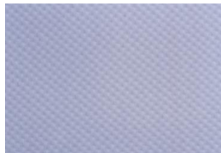
Şekil 2.14. PVC-PES Kumaş (Architectural Membrane Association, 2018)
