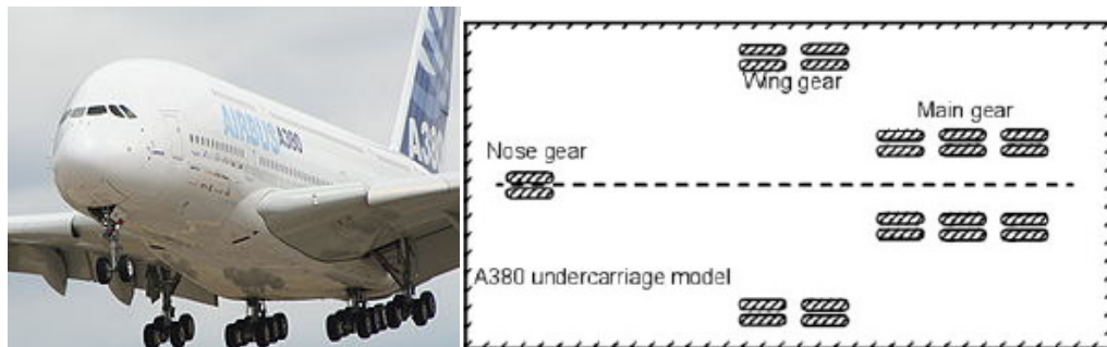
Figure 2.5: a. Airbus A380 landing gear[9]. b. Airbus A380 wheel arrangement [8].
