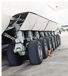
Figure 2.6: Main landing gear of Antonov 225 [9].
