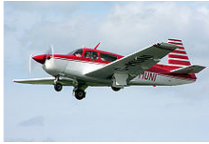
Figure 2.2: Tricycle landing gear of a Mooney M20 [9].
