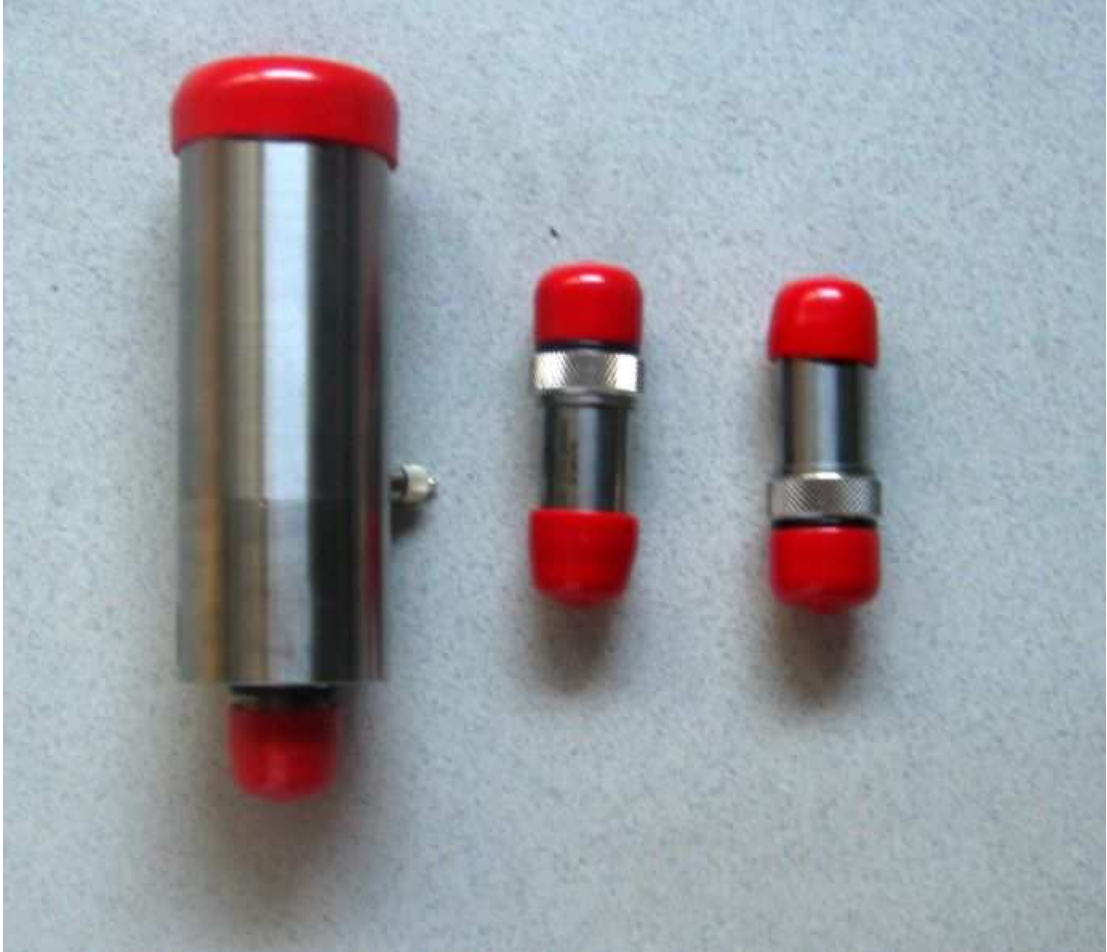
Figure 1.8. Transducers of 50 MHz, 10 MHz and 3.5 MHz.
