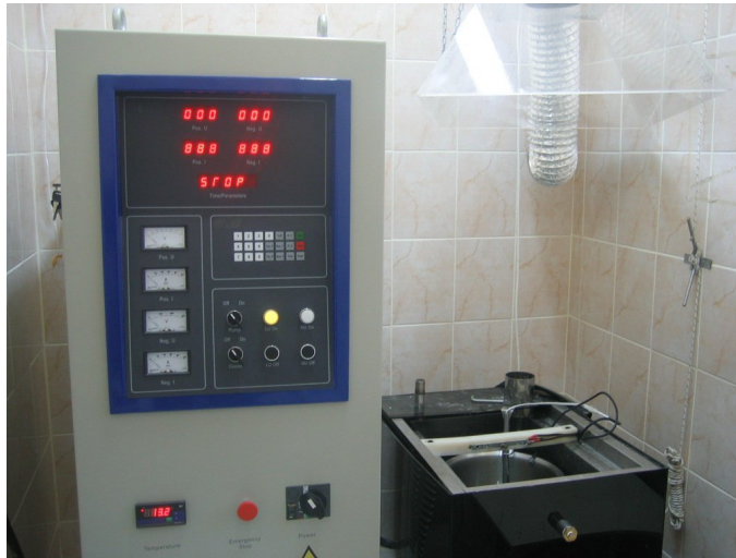
Figure 5.1: Micro-arc oxidation apparatus [57].
