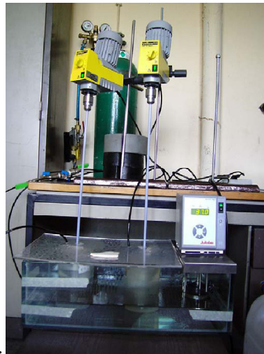
Figure 5.2: Bioactivity test apparatus [54].
