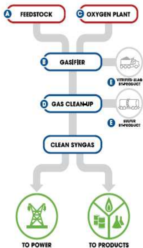
Figure 2.4: Gasification process (Url-1)
