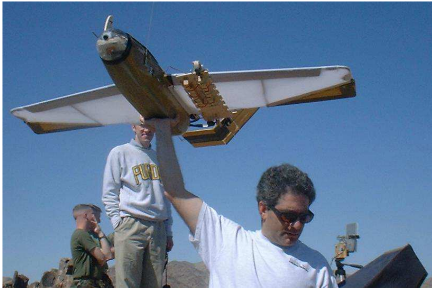
Figure 1.1. The UAV with the sensor node under its wing to be deployed [1].
