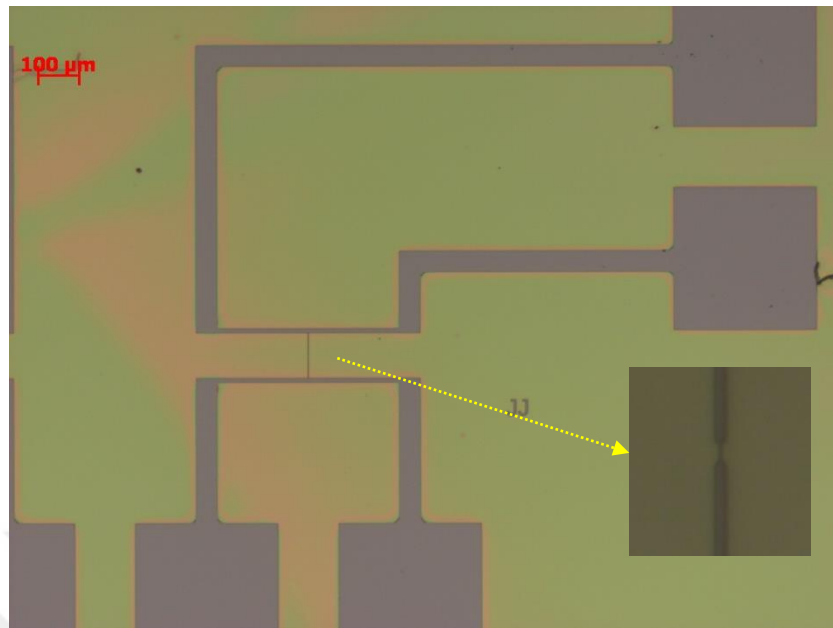
Figure 2.5: Microscope image of the substrate after developing process. Lighter green color shows the resist, darker gray colors show the areas that the resist is removed.
